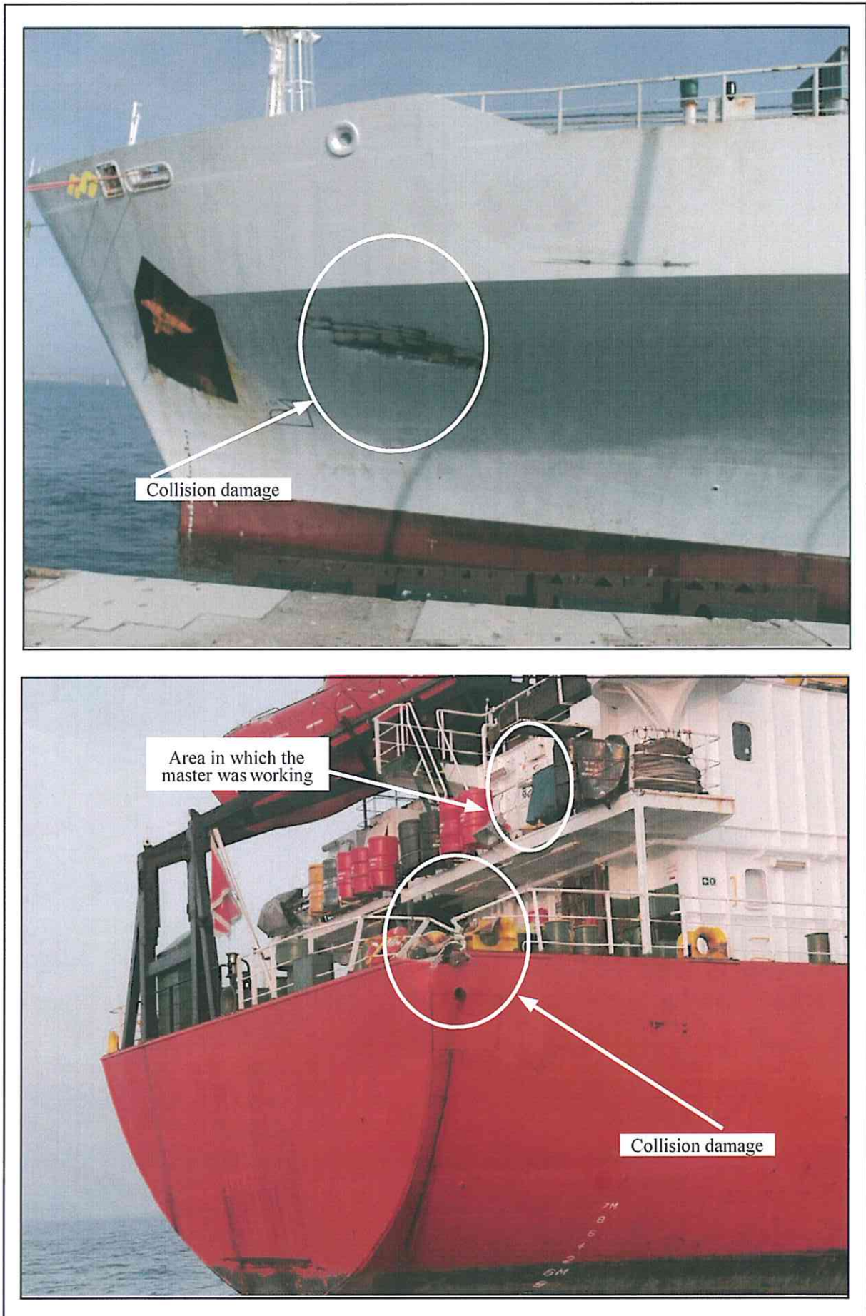
Figure 1: Damage to both vessels
